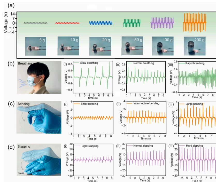
Figure 14. The characteristic output signal of the sensor: (a) under different weight pressure; (b) breathing at different frequencies; (c) bending fingers at different angles; (d) slapping at different strengths. Reprinted with permission from [144]. Copyright 2023 Elsevier Ltd.
