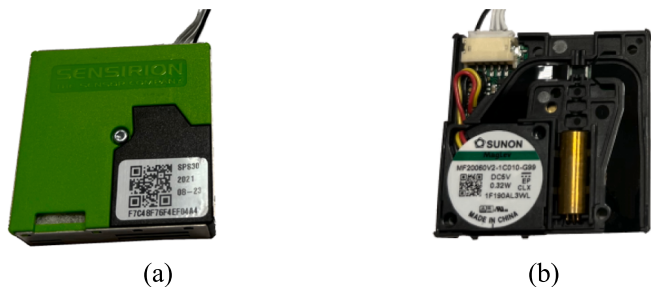
Fig. 1. Low-cost PM sensor SPS30 from Sensirion [60]: (a) top view, (b) sensor's internals.
