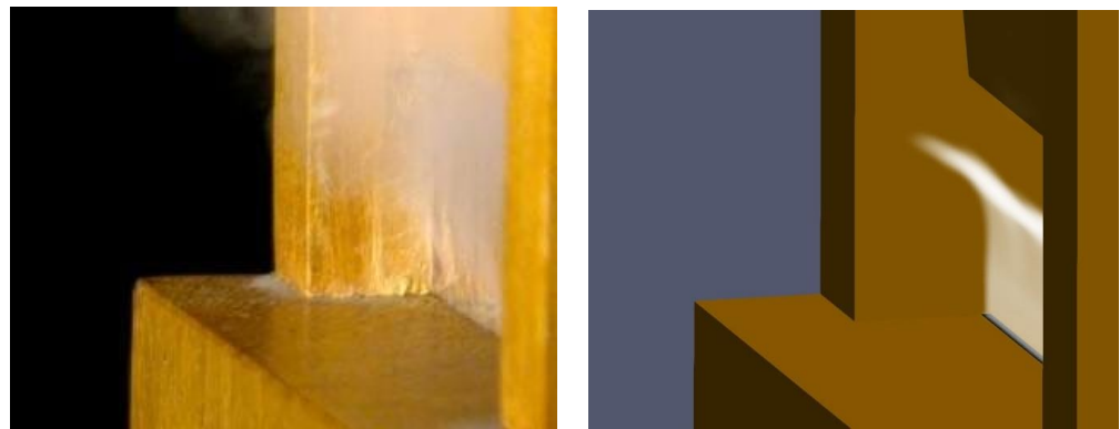
Figure 11. Still images of the jet displacement from the side perspective: HSC frame (left side); numerical simulation (right side). (See the YouTube link: https://youtu.be/WlrITKOpdFo (accessed on 9 March 2024) to observe how the air jet is built).
