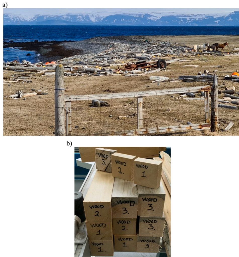
Fig. 1. The investigated driftwood: (a) the Arctic driftwood on the coast of North Iceland; (b) derived experimental samples: WOOD 1 – samples Siberian larch, WOOD 2 and 3 – samples Scots pine.
