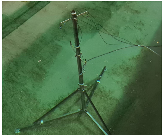
FIGURE 2. Receiving transducers on a mast at the bottom of the towing tank.
