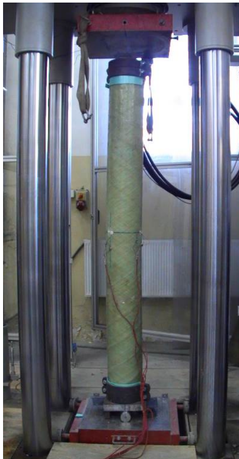
Fig. 3. Composite-concrete column during the test (compression in the press) [10]
