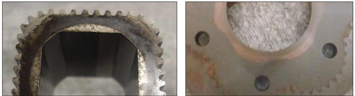
Figure 29. A layer of burnt rapeseed oil on the rotor surface (left) and the characteristic purple layer on the commutation plate (right) —after 3237 min of operation.
