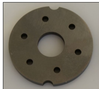
Figure 5. Commutation (compensation) plate of the satellite motor.
