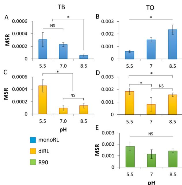
**Figure 3.** Influence of pH on the efficiency of micellar solubilization, expressed as molar solubilization ratio (MSR) for TB (A, C) and TO (B, D, E) in solutions of monoRL (A, B), diRL (C, D) or their mixture (R90) (E). \* $P < 0.05$ , by ANOVA; NS,  $P > 0.05$ , by ANOVA.
