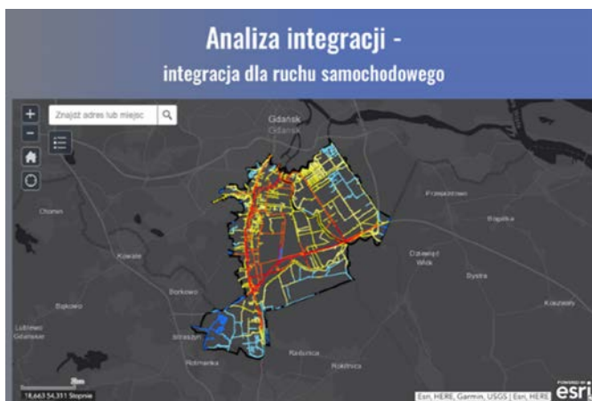
Figure 4: On-line map showing space syntax analysis demonstrating integration analysis for car traffic in the Orunia district of Gdańsk (source: https://infrastrukturagdansk.wixsite.com/mojastrona ) (authors: A. Dziatko, J. Płoski and T. Sitkowski, students, 5th semester of the Spatial Development Programme).
