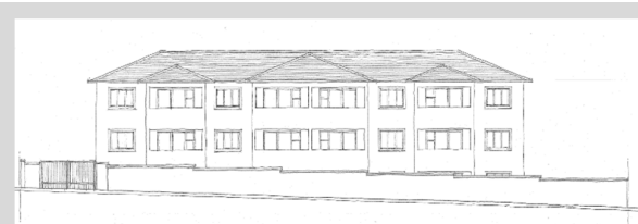
Figure 4-11 - 242 on Brand Road (242 Brand Rd) is one of the most recent developments in the overall study area. It is an exercise in 'reduction' including that of balconies to almost unusable depth. There is a mirror of this form along the sites long axis and the space between is asphalted over with shade cloth car-ports constructed for parking purposes. The solid boundary wall is original, with the electric fencing topping added very shortly after construction.
