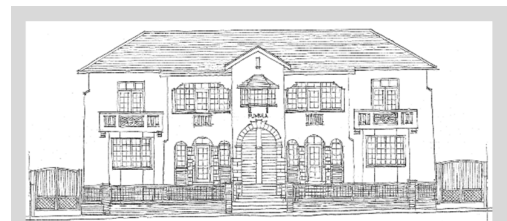
Figure 4-4 - Phumula (64 Hunt Rd) is an exquisitely detailed and maintained Union Period maisonette. Of interest is that there are separate open staircases in the centre of the composition to the two upper floor units.
