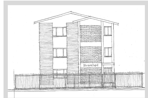
Figure 4-9 - Evershed (89 Hunt Rd) is one of a number of Late-Century Modernist Apartment Buildings in the overall study area. It utilises the contrasting face brick and plaster wall panels, but also uses the face brick breezeblocks for screening elements to external staircases, walkways and in constructing balustrade walls. Double pitched clay tile roofs and standard individual steel window configurations become the standard for these buildings. It still utilises the slope to include parking beneath the building (not visible in the street elevation). The Palisade fence is a far more recent addition, as per the majority trend of constructing subsequent physical barriers along the boundary in the study area.
