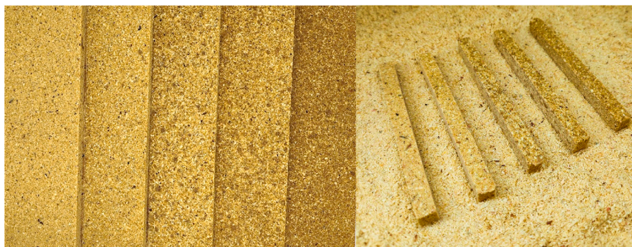
Fig. 2. Manufactured polyurethane-wood composites (from left PU-WC 0% Bio; PU-WC 20% Bio, PU-WC 40% Bio, PU-WC 60% Bio, and PU-WC 80% Bio).
