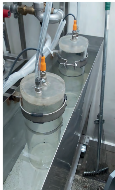
Fig. 3. Biogas collecting vessels with gas throughput sensors
