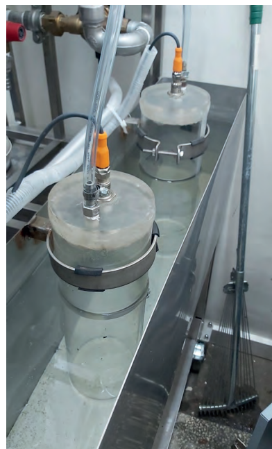
Fig. 3. Biogas collecting vessels with gas throughput sensors
