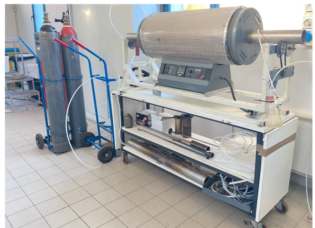
Fig. 2—Self-designed shaft furnace.
