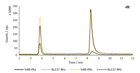
parameters, such as inductively coupled plasma power, torch position, and voltage applied to extraction and focusing lenses, were optimized daily. Hydrogen was used as a reaction gas to reduce spectral interferences. Analytical blanks were run in parallel. External calibration using 12-point calibration curves for metals of interest was used.
