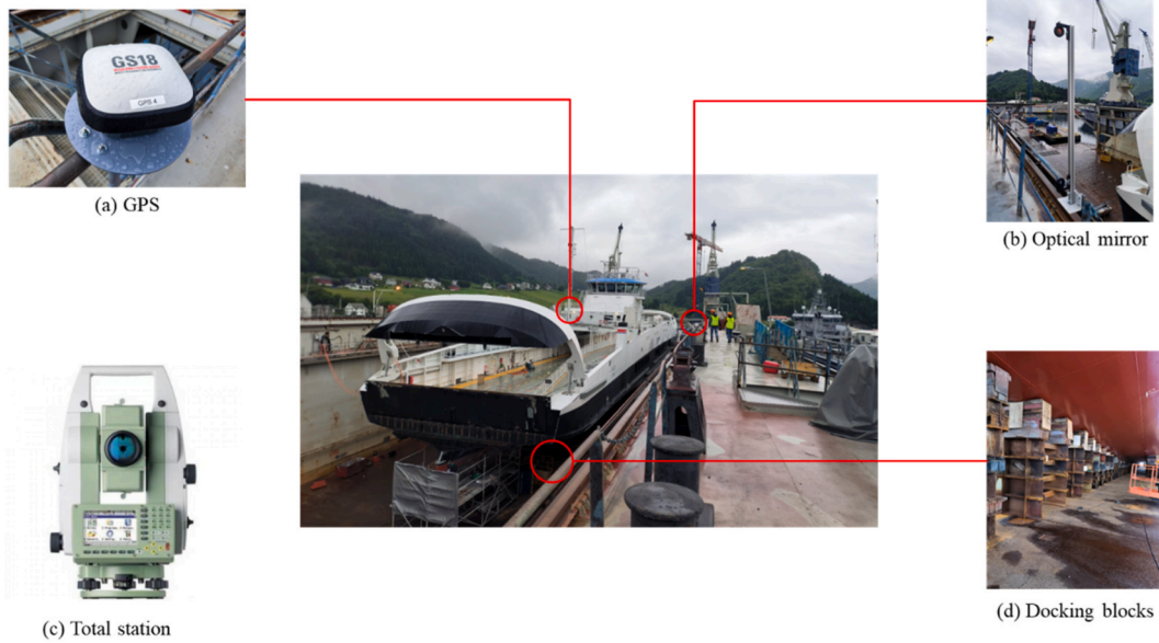
Fig. 24. Setup of field test measurement.
