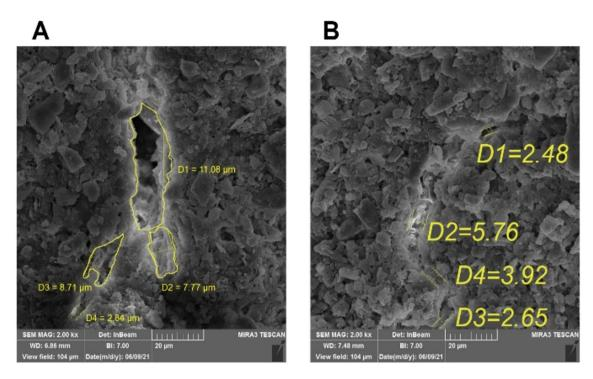
Fig. 4. SEM Images, the sample of mortar sprayed with the NB4-2 Nanoclay solution before and after performing the rain simulator test with a magnification of  $20 \mu m$  (A, B).
