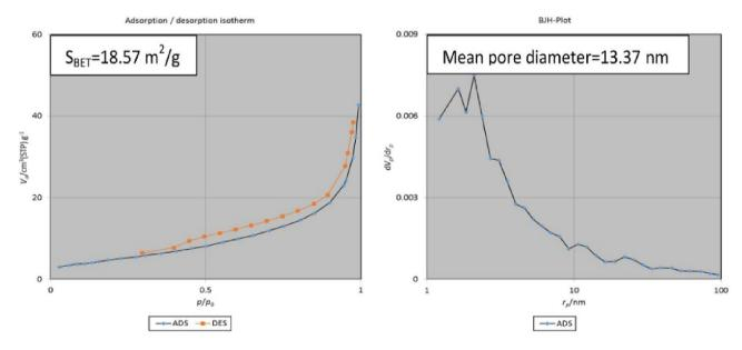
**Fig. 3.** The BET and BJH curves of the NB4-2 sprayed sample.
