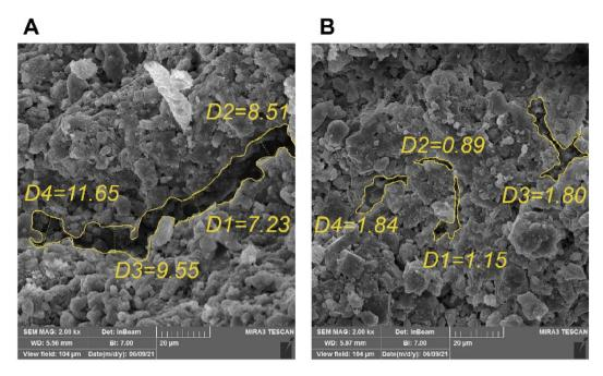
Fig. 6. The effect of accelerated aging Test. Control sample after performing the accelerated aging test with a magnification of  $20 \mu m$ . (A) The mortar sample sprayed with the optimal percentage of NB4-2 Nanoclay solution after performing the accelerated aging test with a magnification of  $20 \mu m$ . (B).
