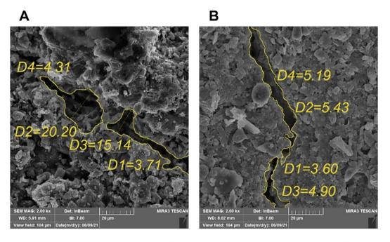
Fig. 5. The effect of freezing on samples. Control sample after performing the frost resistance test with a magnification of 20  $\mu$ m. (A) sample sprayed with the optimal percentage of NB4-2 spray after the frost resistance test with a magnification of 20  $\mu$ m. (B).
