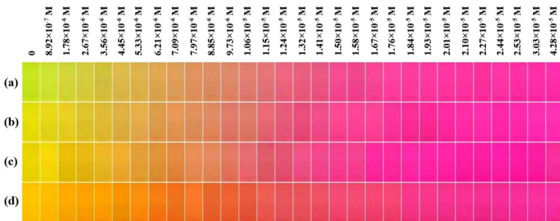
Fig. 18. Color changes of L ( c_L = 2.16 \times 10^{-5} M) upon titration with copper(II) chloride ( c_{Cu} = 0-4.28 \times 10^{-5} M) in water-DMSO (9:1, v/v) solvent mixture at pH: (a) 5.0; (b) 7.0; (c) 9.0 and (d) SBF:DMSO (9:1, v/v) at pH 7.4.
