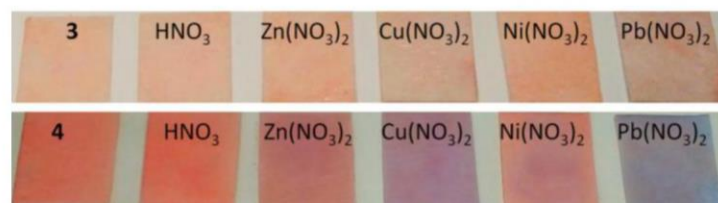
Figure 10. Changes of the color of test strips (glass filter) with adsorbed crowns 3 (2.9 × 10 -4 M) and 4 (3.1 × 10 -4 M) after immersing them for 15 s in solutions of (from left): deionized water, nitric acid (10 -1 M) and metal nitrates (10 -2 M) at pH 5.
