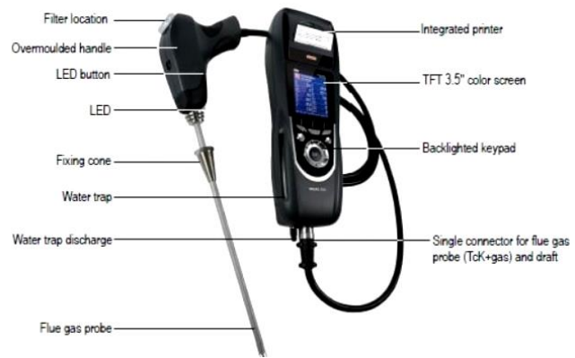
Fig. 3. View of the KIGAZ 300PRO flue gas analyzer used in laboratory tests
