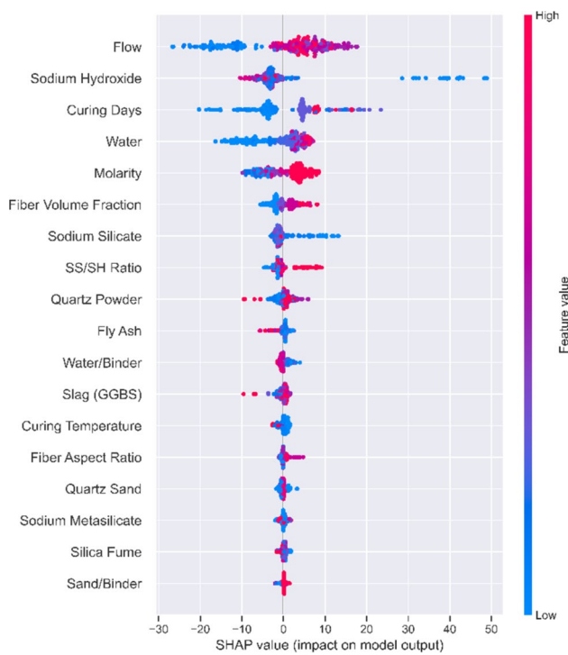
Fig. 5 SHAP global interpretation on compressive strength of AA-UHPC, SHAP value impact on the model
