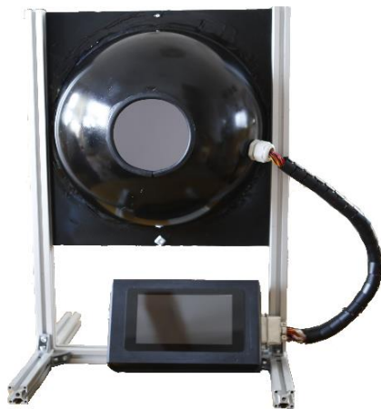
Fig. 6. External view of the mechanical structure of integrating sphere-based lamp with control panel.
