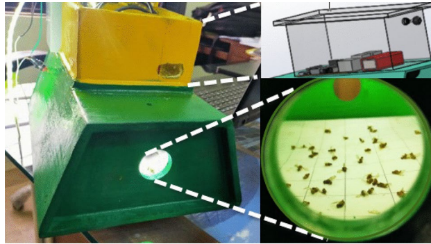
Fig. 3. Intelligent smart trap system which performs Machine Learning-based pest detection at edge device and transmits findings to stakeholders via the cloud and includes a solar-powered IoT-enabled smart insect trap.
