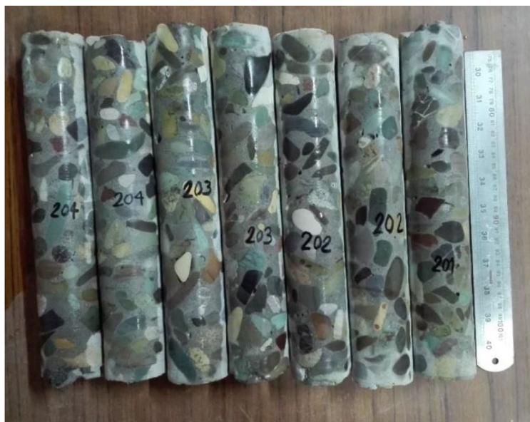
Fig. 4. Samples prepared for a triaxial experiment whose mosaic form is completely clear.
