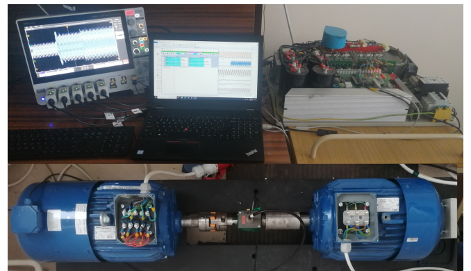
Fig. 12. Laboratory stand with 5-phases induction motor (left) and induction motor emulated the load (right).
