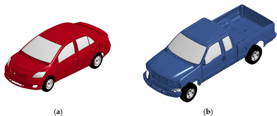
Figure 1. FE models of MASH-compliant test vehicles: (a) A 2010 Toyota Yaris passenger car (1100C) and (b) a 2006 Ford F250 pickup truck (2270P).
