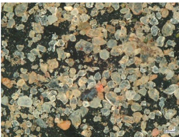
Fig. 5. Microscopic photo of solid particles of mineral origin used during the tests
