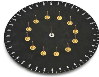
Figure 6: ESPAR antenna used in measurements
