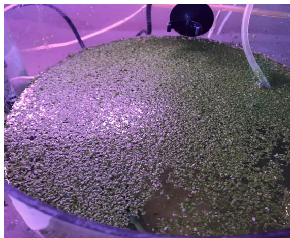
Fig. 1. Phytobioreactor with higher aquatic plants Lemna minor .
