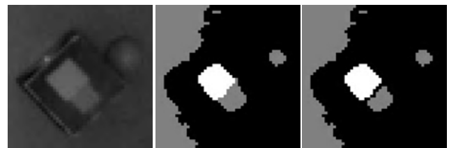
Fig. 7. Grey color threshold and segmentation (a) original image (b) grey color threshold (c) grey color threshold with an extra neighborhood condition.
